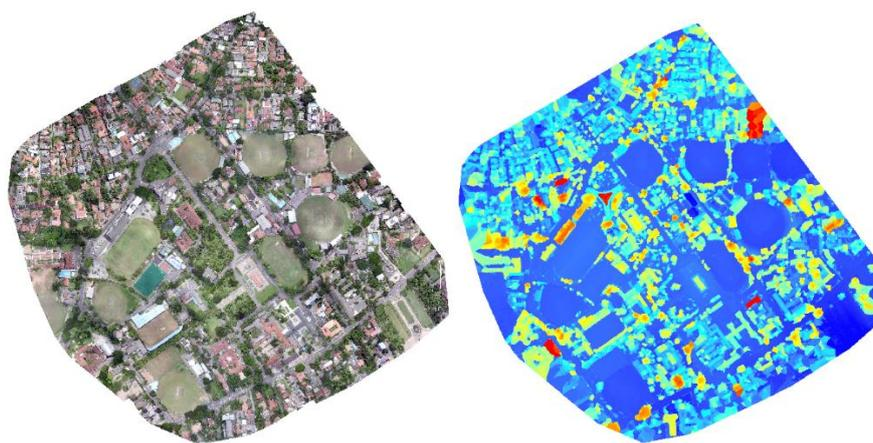
Figure 4. Orthoimage (left) and DSM (right) created by images from Phantom 3
